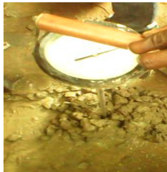
Plate 3: Determining Concrete Temperature
